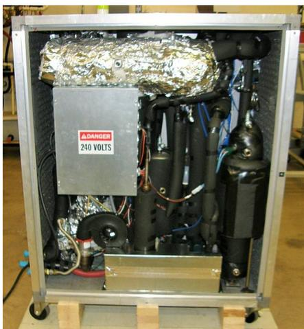
**Figure 2:** Heat pump components housed within unit
